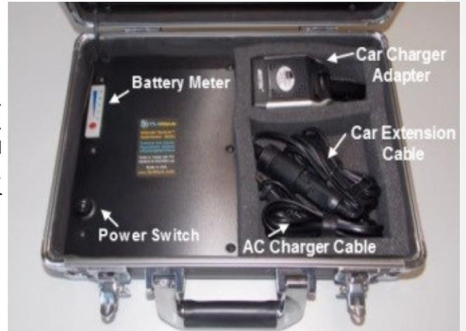
**6 CHARGE INDICATOR LED** - The unit has a charge LED (see photo). This is a two color LED. It will be green when the battery is ON (faint to conserve battery). It will be red (or blinking red) when the battery is being charged. When charging, the red LED will turn green when the battery has completely charged.
