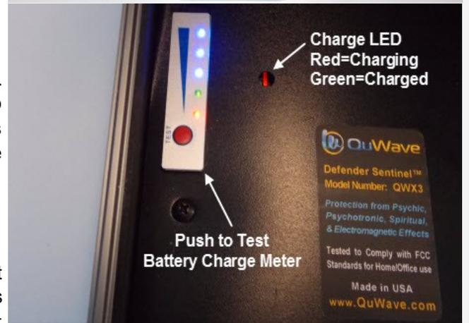
**7. CHARGING TIME** - Depending on the state of the battery, it might take between 2-5 hours to completely re-charge. Many customers charge the unit overnight. Also included is a Car adapter which allows it to be charged from your car.
